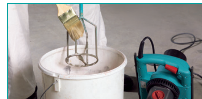
Easy cleaning of the mixing tool for greater effectiveness and longer service.
